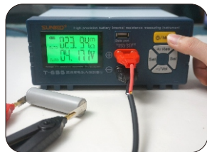
Measure the 18650 battery: IR:23.94mΩ, V:4.17V.
