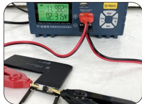
Measure the battery of Iphone: IR:11.982mΩ, V:2.315V.
