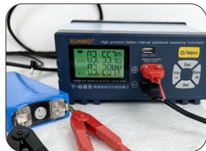
Measure the lithium iron phosphate battery: IR:3.557mΩ, V:3.284V.
