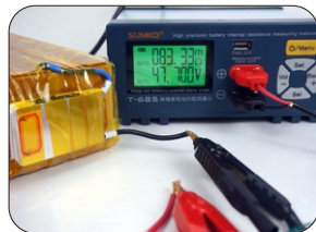
Measure the 13S 48V 18650 battery pack: IR:83.33mΩ, V:47.7V.
