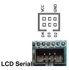
This shrouded header provides D2-D4 along with power and ground for connecting to a serial LCD display.
