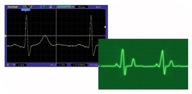
The ECG pulse of the FG-050 compared to the ideal pulse. (© 2018 Jos Verstraten)
