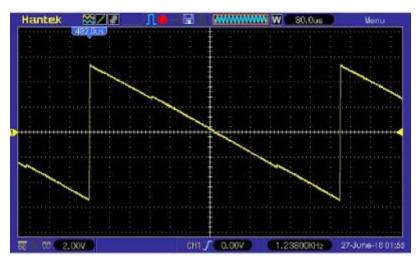
*Test of the linearity of the DAC by generating a sawtooth.* (© 2018 Jos Verstraten)
