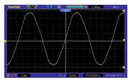
The maximum sine wave signal at the maximum frequency of 65.534 kHz. (© 2018 Jos Verstraten)
