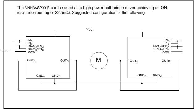
Figure 13. Multi-motors Configuration
