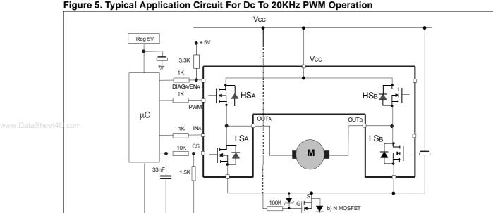
Figure 5. Typical Application Circuit For Dc To 20KHz PWM Operation
